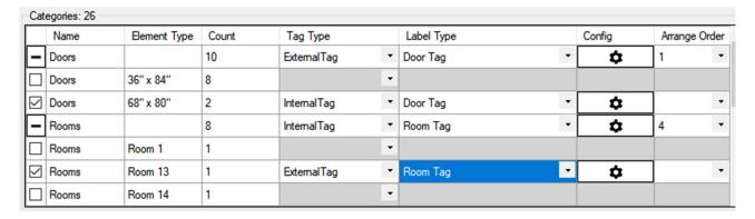
By checking the selection box next to the type, it is enabled, allowing a specific configuration; in the absence of changes to the type, the standard configuration chosen for the category will be applied.
