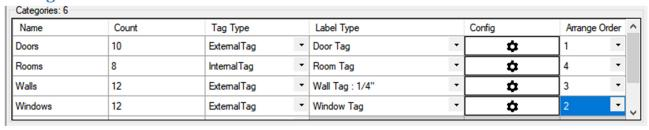
It contains information on the categories of elements present in the view and allows their configuration for the tagging operation.
