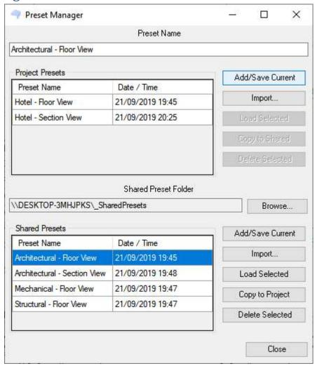
It allows to quickly define the set of configuration settings to be used for the tagging operations of the various types of view. These operations are normally performed by the project manager (or studio manager for shared presets).
